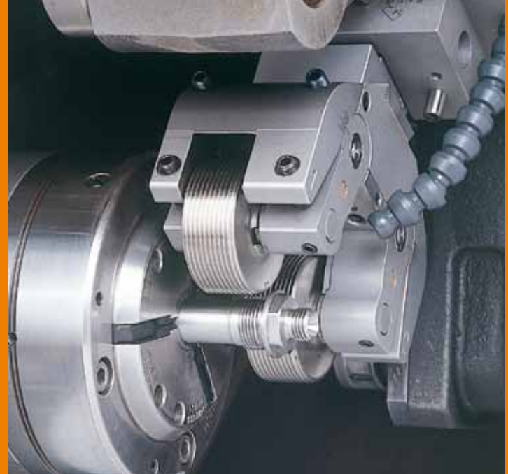
Thread rolling behind a collar
