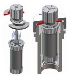
Schaublin presents a new solution for the internal clamping of parts. Instead of inserting the F-type collet, simply insert the expanding arbor, that's it. There is no adjustment required for the seating and no other accessories are required. The interchangeable sleeve is pre-machined and soft to allow an easy adjustment to various clamping requirements. The presented F38 type is capable of internal clamping in the range of ø20 to ø38 with lengths up to 26 mm.
