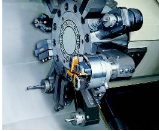
Head ZA 22 on CNC lathe with disk revolver
