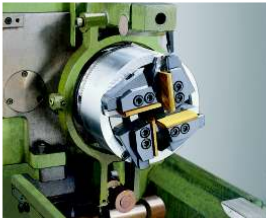
Head Z 39 on thread cutting machine
