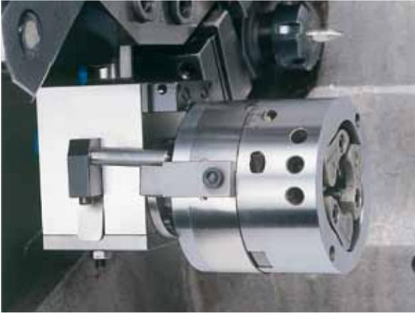
**Stationary RS16 rolling head with locking device**
